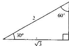
$$30^\circ = 30^\circ \left( \frac{\pi}{180^\circ} \right) = \frac{\pi}{6} \text{ radian}$$
